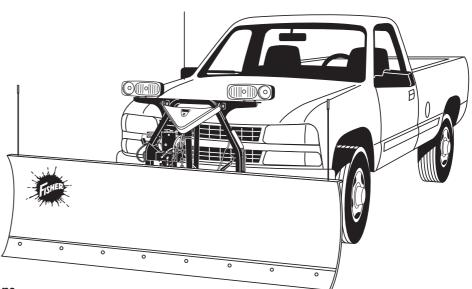
Accessories include a steel cutting edge made of 1084 high carbon steel to improve cutting power and scraping ability, the FISHER® SnoFoil® to funnel snow to the side, curb shoes and a Plow Parka which fits over the lights and headgear for protection from the elements. A steel or 2-ply rubber deflector is also available to help keep snow off your windshield.
